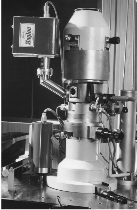
FIGURE 38 Électrocomposeur with its LaB6 gun in service in 1975 at the semiconductor factory of Saint-Égrève, near Grenoble.
